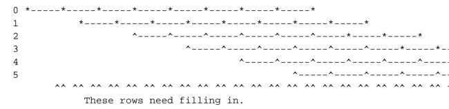
In this case, the first J - (J/G) = 9 - (9/3) = 6 jets of pass p + (6/3) = p + 2 collide with the last 6 jets of pass p. Only one row in every G = 2 rows is printed by this weave.
